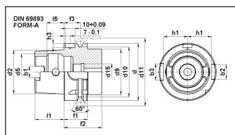
Standard type for use on milling machines and machining centres with automatic tool change. Also suitable for manual tool change.
